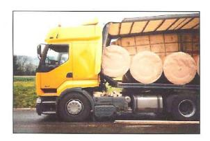
Loads should be restrained so that they can't move independently of the trailer.
