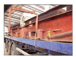
Webbing straps should be checked regularly for damage. Even a small cut or tear can reduce the strength of the strap significantly.
